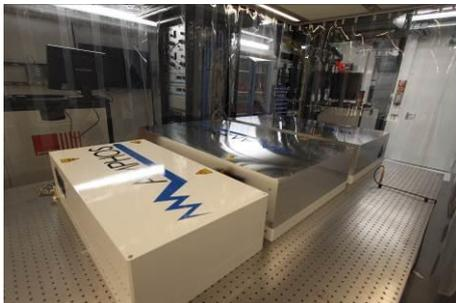
Foto: 5kW Amplifier Chain installed at XFEL lab at SASE 1 beamline
